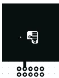
a) 76°C/W when mounted on a 1in<sup>2</sup> pad of 2 oz copper
